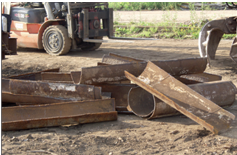
Figure 6: TENORM polluted steel pipes [14]
