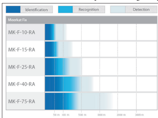
Fig. 8 DRI parameters of a few thermal cameras
